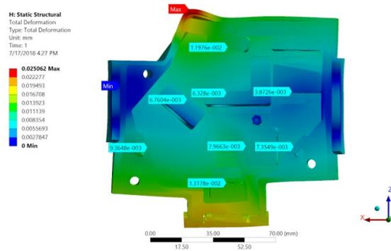
**Figure 4: Modeled deformation due to thermal strain from -10 to 30 C temperature change**
