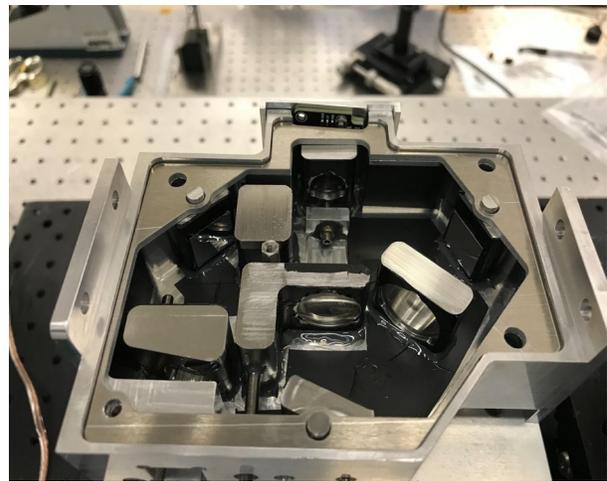
**Figure 3: SPOCeye optical layout and housing showing the 11 optical elements of the system. The entrance pupil is located at the bottom of the image.**
