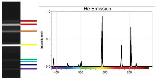
**Figure 5: Left, spectral alignment testing using a Helium source. Right, reference image from Vernier.**
