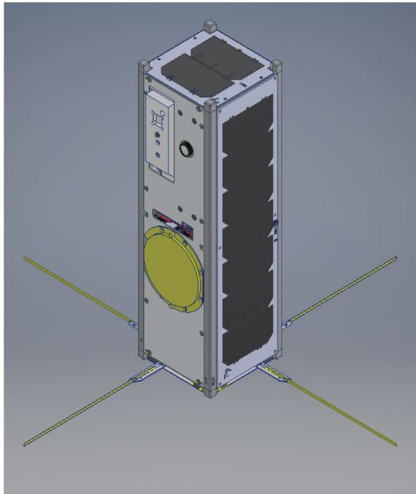
**Figure 2: Current SPOC design, a 3U standard CubeSat with deployable antennas.**
